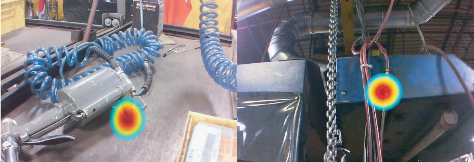
Images taken with the ii900 Sonic Industrial Imager in an industrial environment.
